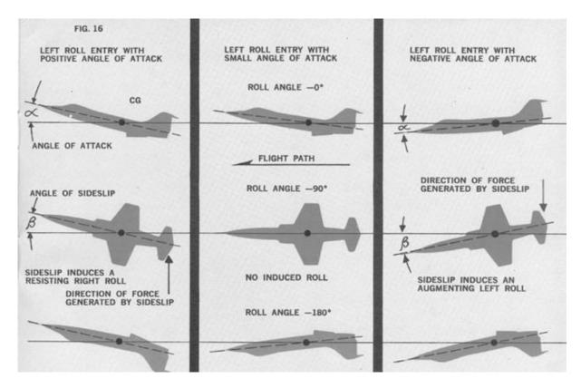
In the second series, the aircraft is being rolled with the angle of attack almost nil. Here we see that no sideslip or additional rolling moments are generated. This is the type of roll we all strive for.
