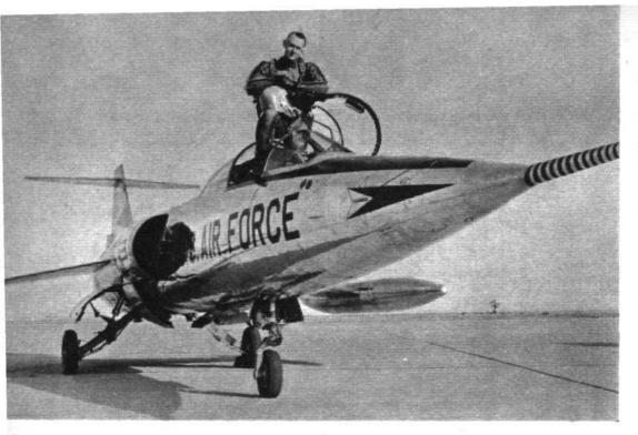
Tony LeVier, Lockheed's director of flying operations and F-104 test pilot, poses in partial pressure suit with a prototype F-104. Production machines have forward-retracting nosewheel, intake shock-bullets, landing and taxying lights, and many other refinements. Span is 21ft 11in, length 54ft 9in and height 13ft 6in.
