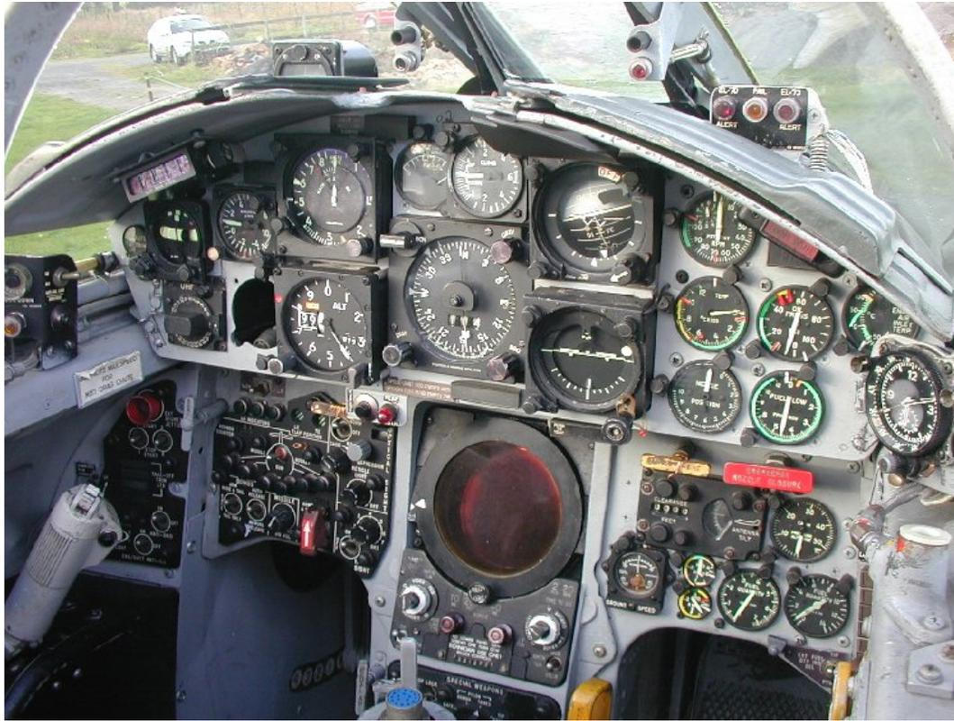
Main, lower and left auxiliary instrument panel of a German F-104G
