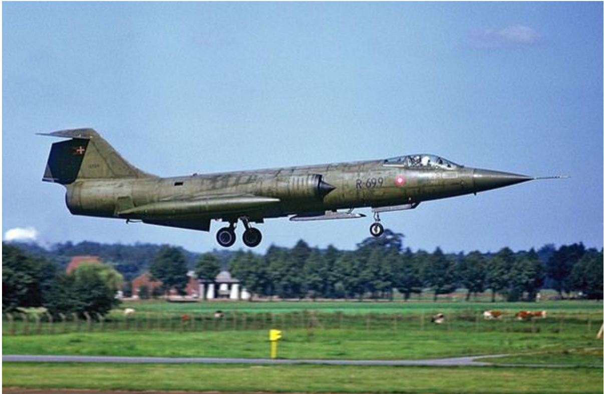
© Wieland Stolze R-699 F-104G Esk 723, Gütersloh (September 1975) One of the four Danish F-104G for the squadron exchange with the 92 Sqn was the R-699, seen here on the final for RWY 09. As in this case, the engine was always kept at a high speed (RPM) in order not to lose the air flow blowing over the wings (BLC). The catamaran carrier under the fuselage were typical of the Danes and German Navy Starfighter.
