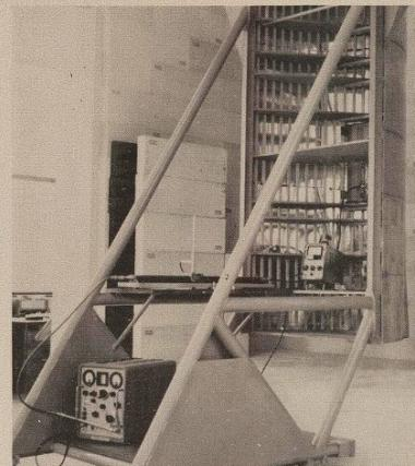
**Antenne testing in anechoic chamber**
