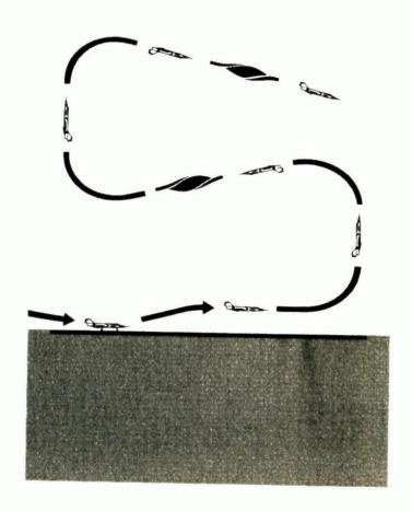
The next maneuver is one that Snake believes can *only* be performed by the Starfighter. He will make a normal approach and landing touchdown. At touchdown he will apply full afterburner for the go-around, but at the far end of the runway he will perform a double Immelmann. The Starfighter is the only fighter in the world that has enough excess thrust to perform a double Immelmann from takeoff attitude.
