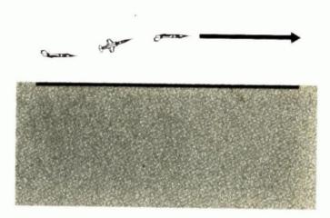
During air combat, a fighter must have the ability to fly in all attitudes in order to be positioned for firing on the enemy. This means that all systems must remain "go" while the fighter is being flown in any attitude. Snake will now demonstrate the ability of the Starfighter to maintain full attack readiness even under the most severe condition — prolonged inverted flight. Following this pass, Snake will turn around for the next maneuver.
