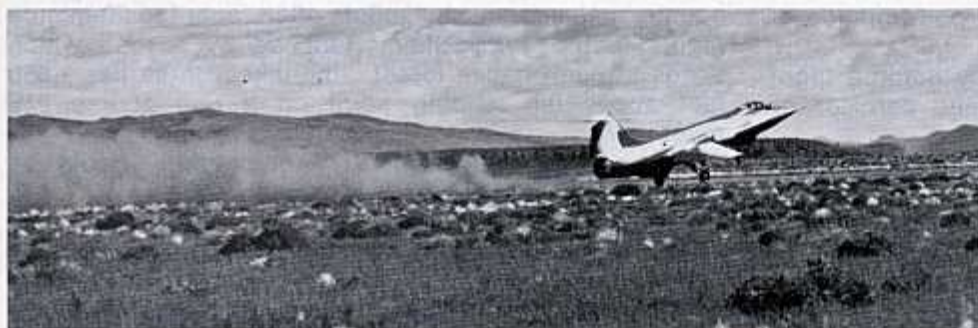
Man and machine break ground after a thundering take-off roll. The GE J-79-10 engine powering the Starfighter produced over 19,000 pounds of thrust—almost exactly a one-to-one ratio with the weight of the plane.
